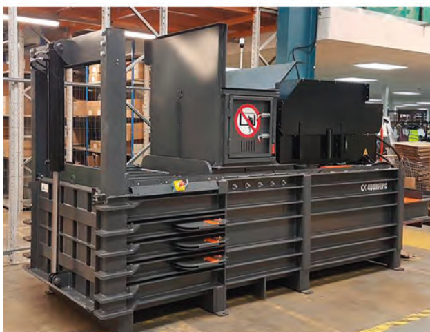
Prensa (H x W x D) 4470 mm x 1570mm x 2220mm Bala (H x W x L) 800 - 1200mm, 1150 x 750mm.
